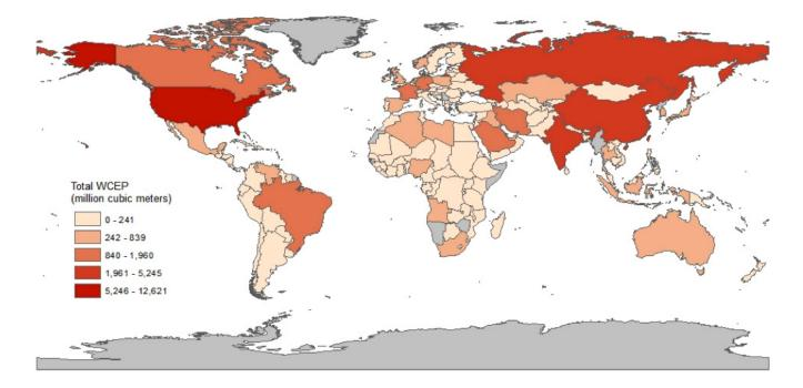
CWEE researchers addressed this knowledge gap by developing a global distribution of water consumption by national-level energy portfolio. We defined and calculated a water consumption for energy production (WCEP) indicator to quantify and compare the water use of 158 national energy systems. WCEP estimates freshwater consumption across all energy categories, including fossil, nuclear, and biofuels, as well as electricity production.
